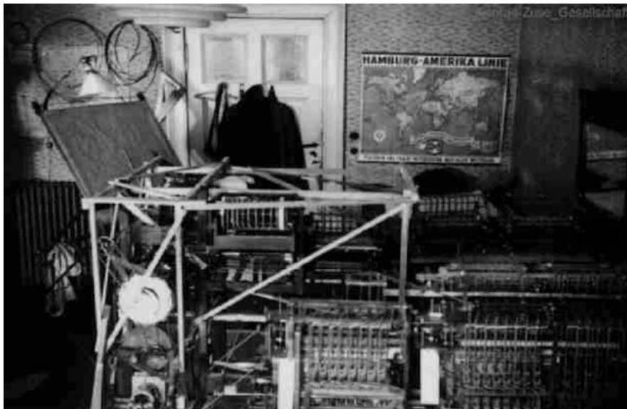
Fig. 1.4 One of the few existing pictures of the mechanical Z1 built in Zuse's living room (Image: Deutsches Museum)
