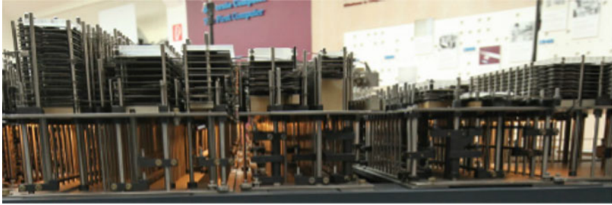
Fig. 3.2 The mechanical layers of the Z1. The eight memory layers can be seen on the right; the 12 processor layers on the left. The lower section with levers is used for transmitting the clock cycles to all parts of the machine ( http://zuse.zib.de )
