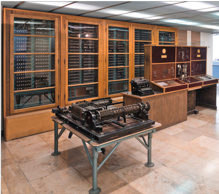
Fig. 8.1 The Z4 at Deutsches Museum. The mechanical memory and the control console are visible in the foreground. In the background, we can see the racks of telephone relays used for the logic components. The two tape readers are visible in the center of the console. The right side of the console is used for entering instructions and addresses. The left side is used for entering decimal numbers, which are displayed in a lamp array similar to the keyboard of a vintage cash register. Results could be printed with the electric typewriter on the left of the console (Image: Deutsches Museum)
