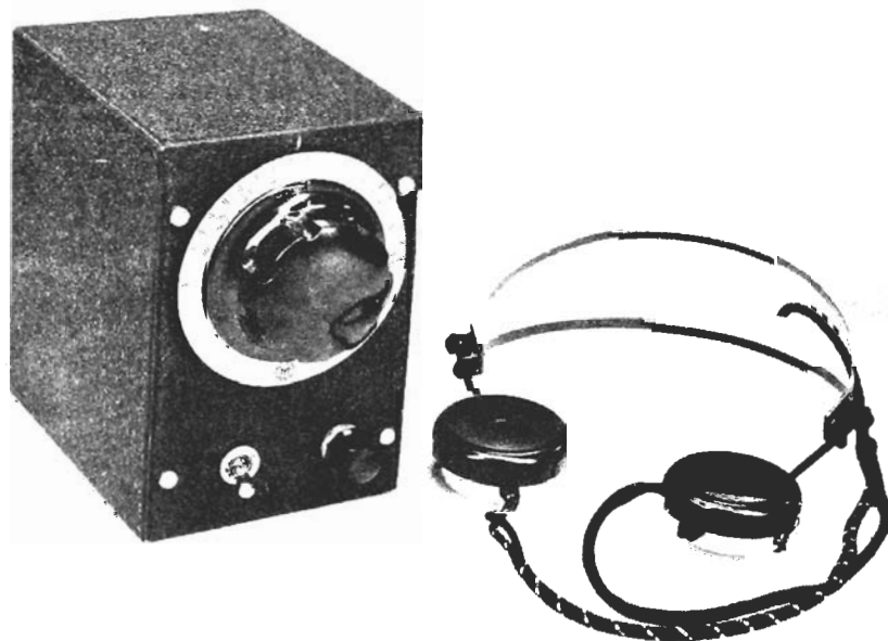
Over-all view of the experimental transistor receiver showing accessory headphones.
