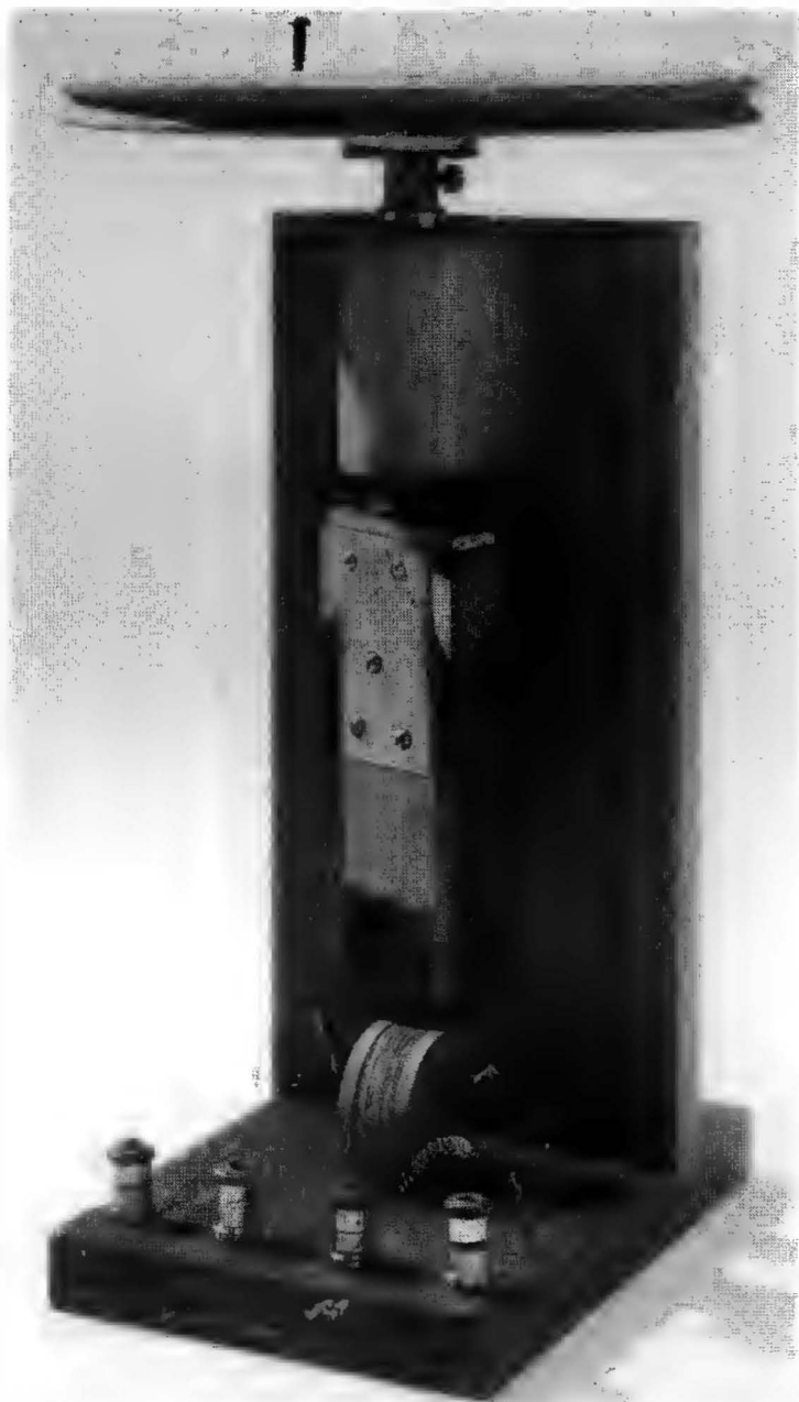
Fig. 5.16 Marconi's first hysteresis detector, which used a rotating permanent magnet [Science Museum photograph]
