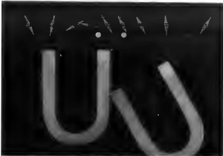
Fig. 5.23 Experimental observation of field configurations in Marconi moving-band hysteresis detector (a) corresponds to Fig. 5.20b (b) corresponds to Fig. 5.20c
