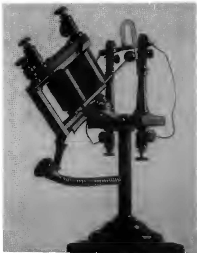
Fig. 3.29 Blondel's side-pocket coherer with its tapper [Collins, Electrical World and Engineer , 39, 1902]
