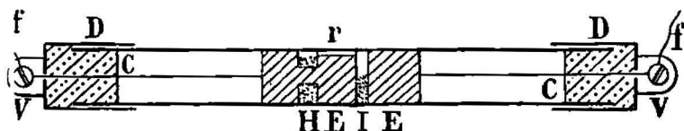
Fig. 3.25 Ferrié's arrangement for adjusting the quantity of filings in the gap By appropriate manipulation, filings could be transferred from the channel H along groove r into the main gap I [Mazzotto, D.: Wireless telegraphy and telephony (Whittaker, 1906), p. 173]
