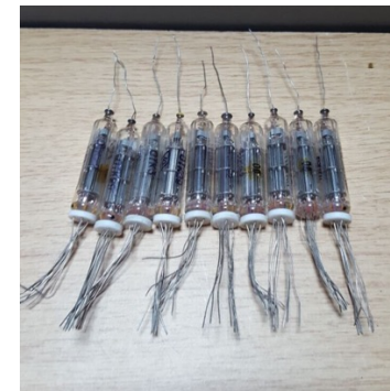
Soviet sub-mini tubes from 1950s
