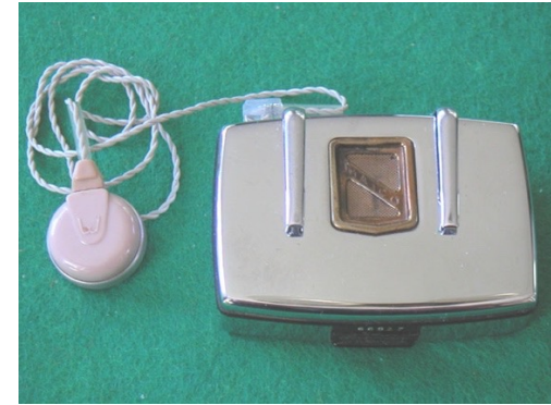
First electronic transistorized hearing aid Used several CK718 transistors
