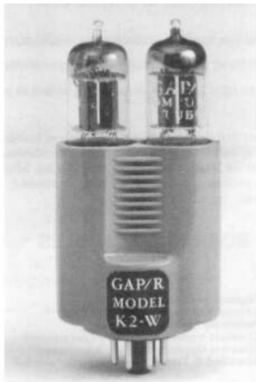
The first commercial Operational Amplifier
