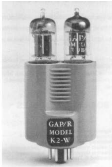
The first commercial Operational Amplifier
