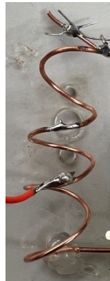
Auto-transformer from Lab 2 radio:
