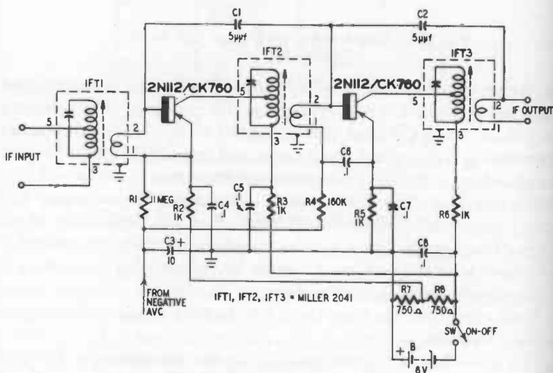
Fig. 203. Two-stage 455-kc if amplifier.
