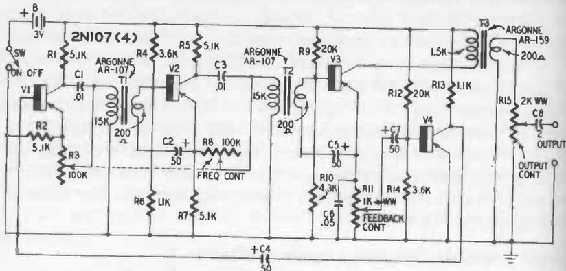
Fig. 406. Tuned variable-frequency audio oscillator.
