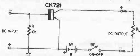
Fig. 302. *Single-stage current amplifier with fixed input resistance.*
