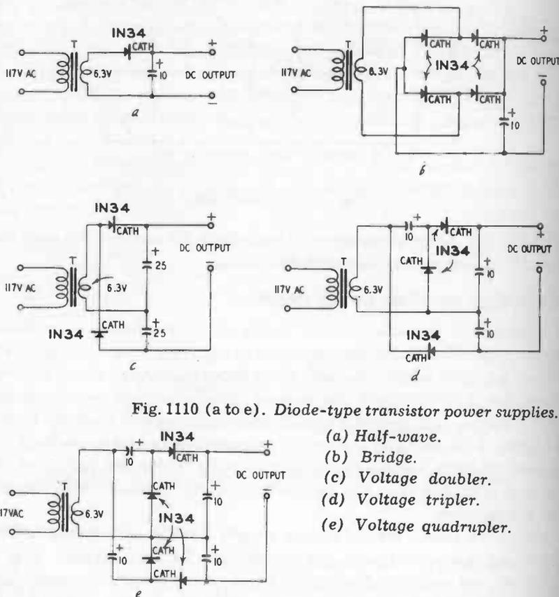
Fig. 1110 (a to e). Diode-type transistor power supplies.
