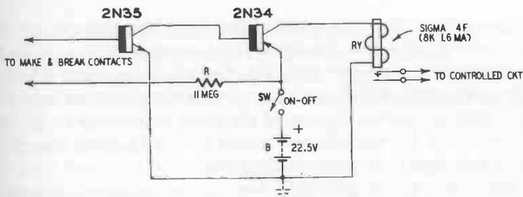
Fig. 803. Sensitive switching circuit for light-duty contacts.
