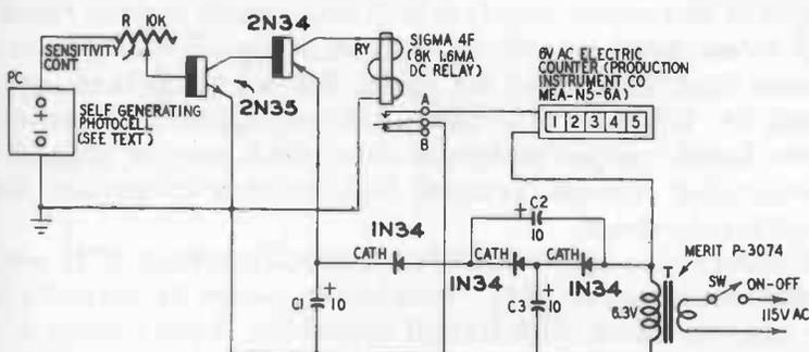
Fig. 811. Photoelectric counter.
