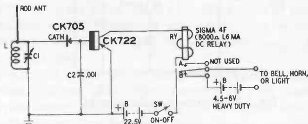
Fig. 815. Carrier failure alarm.
