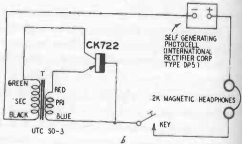
cillators operated from microwatt dc supplies. A typical example is the light-powered oscillator in which the dc collector bias is supplied by a self-generating photocell.
