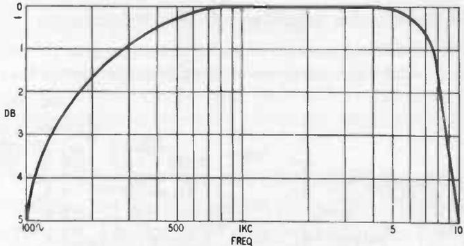
Fig. 118. Frequency response of Class-B loudspeaker amplifier with power transistors.
