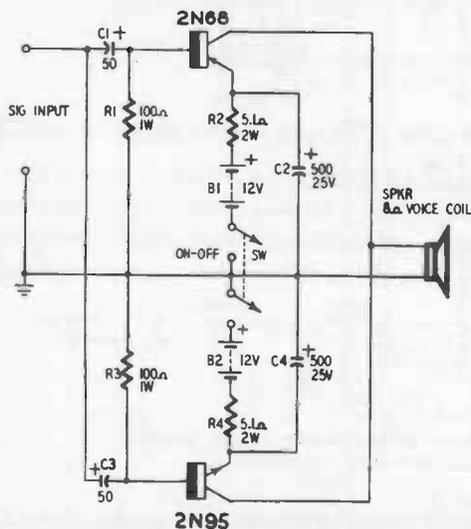
Fig. 121. Complementary-symmetry power amplifier with power transistors.
