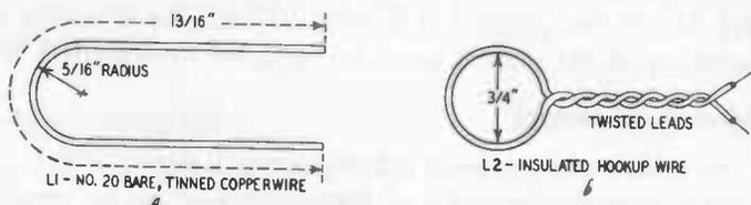
Fig. 912-a, -b. Details of field-strength meter coils.
