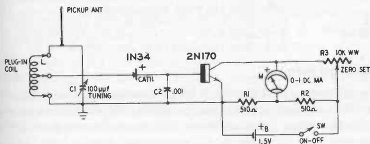
Fig. 1005. Field-strength meter.
