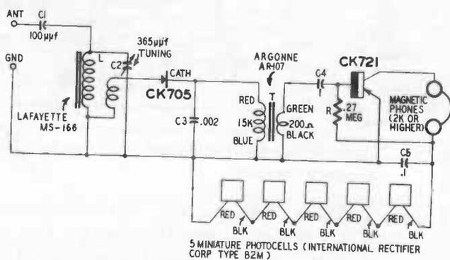
Fig. 608. Sun-powered broadcast receiver.
