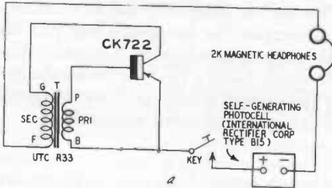
Fig. 414-a, -b. Light-operated oscillators: (a) conventional transformer; (b) subminiature transformer.
