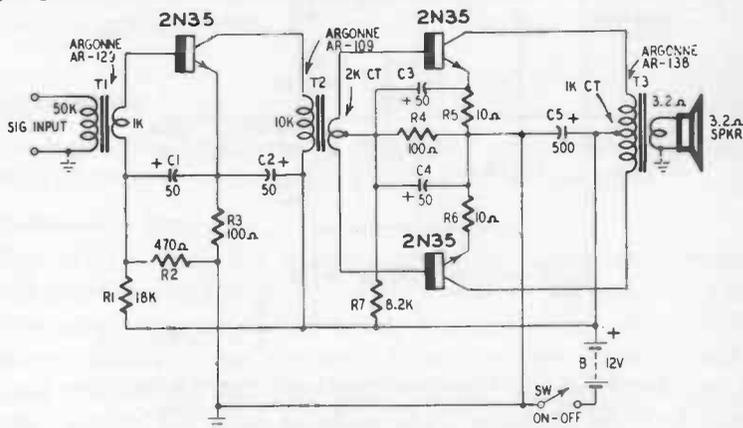
Fig. 116. Class-B loudspeaker amplifier with conventional transistors.
