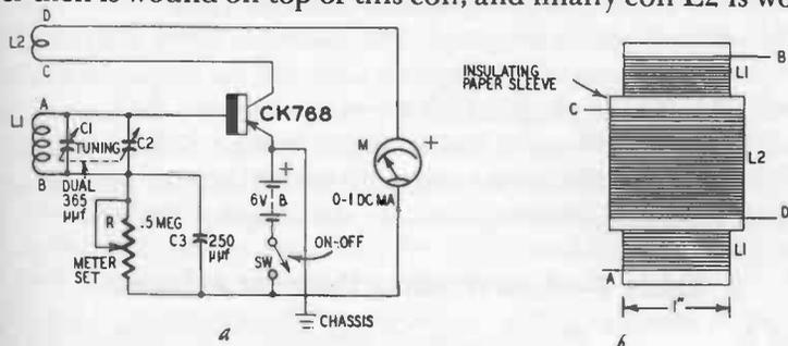
L1: 113 turns No. 32 enameled wire closewound on 1-inch-diameter form.
