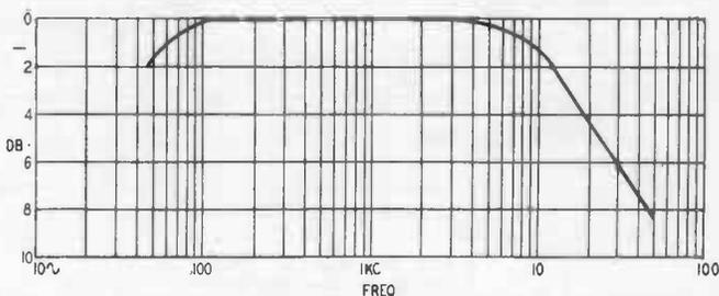
Fig. 106. Frequency response of circuit shown in Fig. 105.
