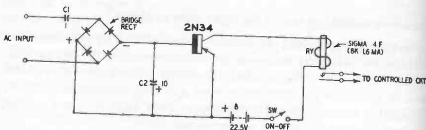
Fig. 804. Sensitive ac relay.
