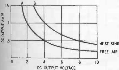
Fig. 504. Performance limits of high-current supply.
