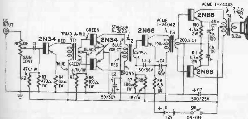
Fig. 117. Class-B loudspeaker amplifier with power transistors.
