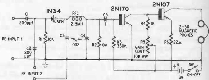
Fig. 919. Radio-frequency comparator.
