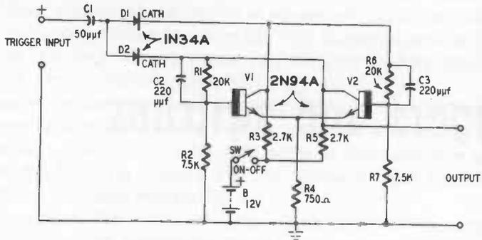
Fig. 701. Flip-flop circuit.
