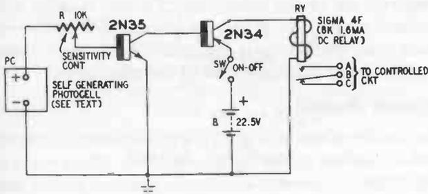
Fig. 810. Light-operated relay.
