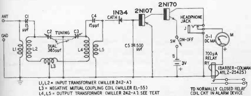
Fig. 1008. Conelrad receiver.
