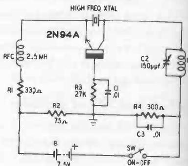
Fig. 409. High-frequency crystal oscillator.
