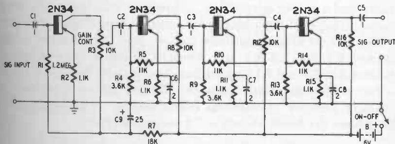
Fig. 111. Multistage R-C-coupled amplifier.
