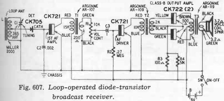
Fig. 607. Loop-operated diode-transistor broadcast receiver.
