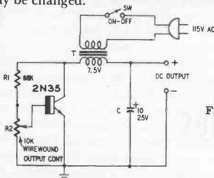
Fig. 501. Variable low-current dc power supply.
