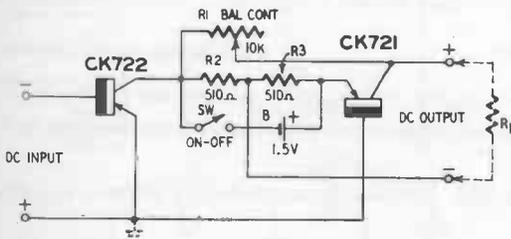
Fig. 304. Cascaded current amplifier with balance control.
