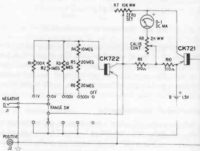
Fig. 906. Electronic dc voltmeter.
