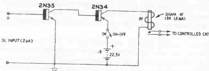
Fig. 802. Ultra-sensitive dc relay.
