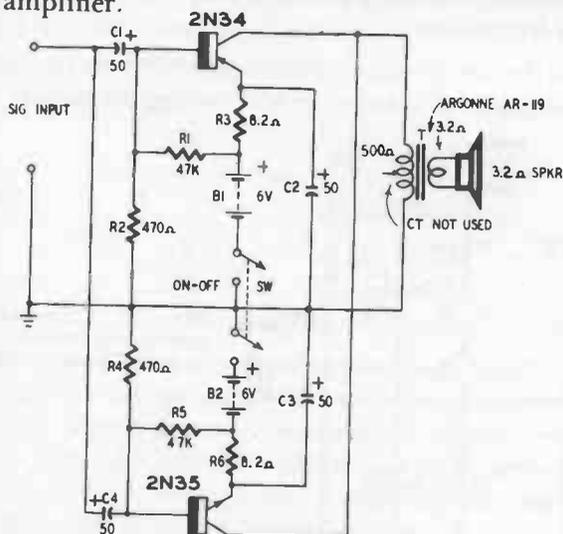
Fig. 120. Complementary-symmetry power amplifier with conventional transistors.
