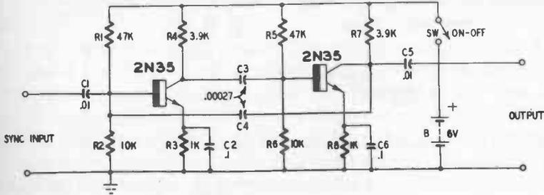
Fig. 412. Multivibrator circuit.
