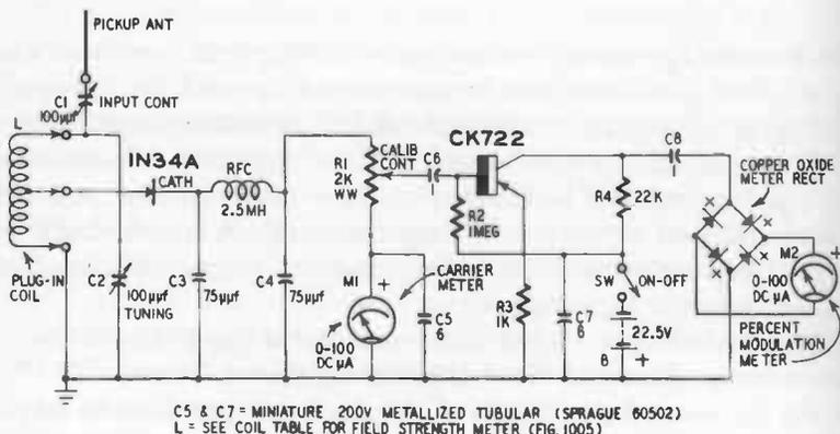
**Fig. 1006. Modulation monitor.**
