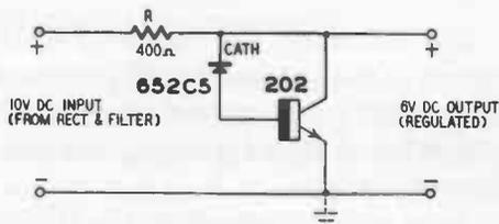
Fig. 507. Light-duty dc voltage regulator.
