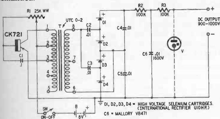
Fig. 513. High-voltage dc-to-dc power supply.
