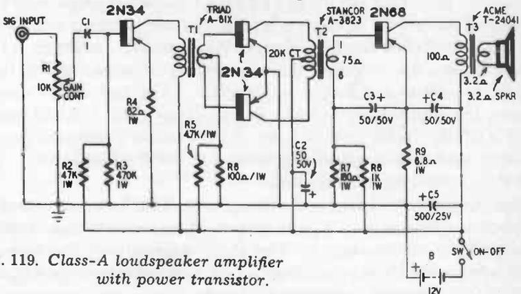
Fig. 119. Class-A loudspeaker amplifier with power transistor.
