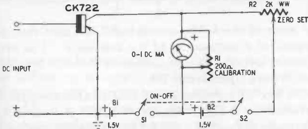
Fig. 902. Battery-type zero-set circuit for microammeter.
