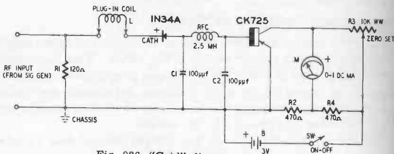
Fig. 926. "Grid"-dip adaptor.
