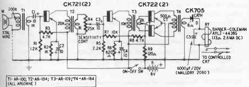
Fig. 809. Sound-operated relay.
