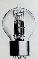
Fig. 6-25. The Type K, or 202A vacuum tube. This is an early version with a machined brass base.
