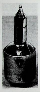
Fig. 17-6. A later Donle tube without the stabilizing enclosure and equipped with a UV base.
