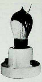
Fig. 4-3. Fleming valve made for C. D. Babcock by McCandless & Company in latter part of 1905.
