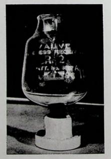
Fig. 11-19. Osram R2A valve fitted with a candelabra base for use in British naval apparatus designed to use the de Forest Audion. This valve was usually supplied unbased; the user applied whatever base he required. Before leaving the consideration of soft values of British origin, mention should be made of the so-called NPL value, described by Stanley in 1919 as follows:
