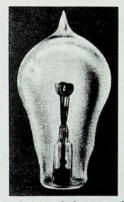
Fig. 12-11. First high-vacuum tube produced at the incandescent lamp factory of Siemens & Halske. (Reproduced from Arch. Gesch. Math. Naturwiss. Tech., 1931.)
