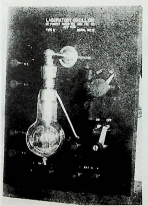
Fig. 7-3. The Type S Oscillion. (Reproduced from *Elect. Exper.*, Apr., 1917.)
