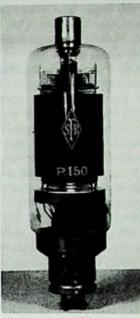
Fig. 19-18. SFR P150 transmitting tube.
