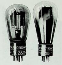
Fig. 16-19. Radiotrons UX280 and UX281.
