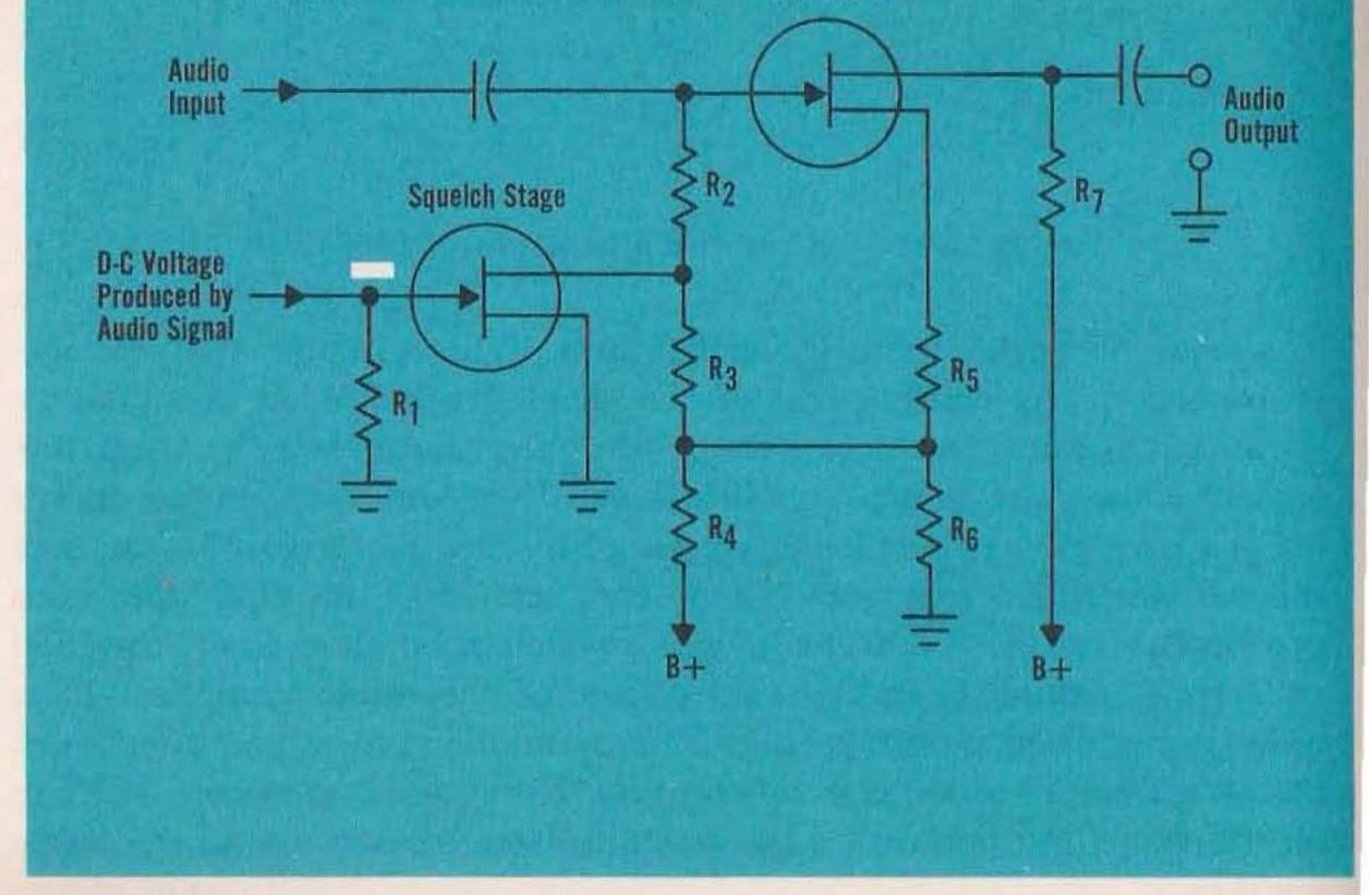
In between stations, when the negative voltage is not there, the squelch stage conducts heavily, putting the junction of R<sub>2</sub> and R<sub>3</sub> at a low voltage (near ground). This cuts off the audio amplifier
