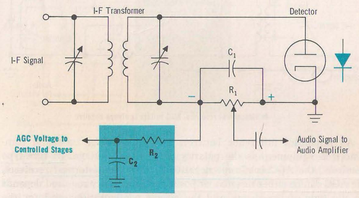
R<sub>2</sub> and C<sub>2</sub> make up an audio filter
