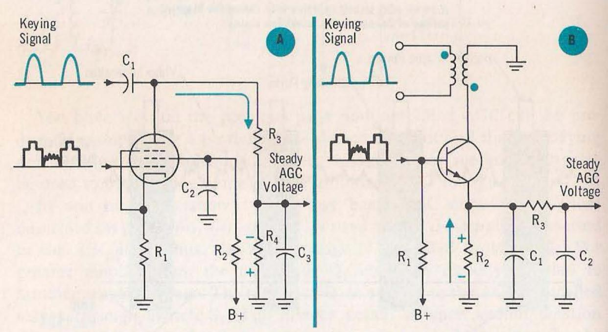
In keyed AGC circuits, the AGC voltage is produced only during the time that the keying signal is present. The average current that flows depends on the amplitude of the blanking pulse
