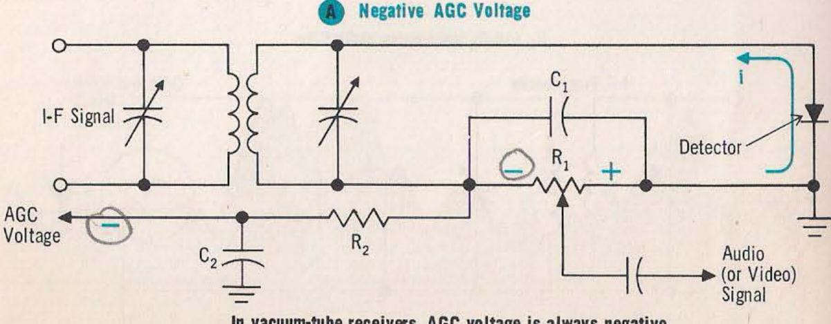
In vacuum-tube receivers, AGC voltage is always negative
