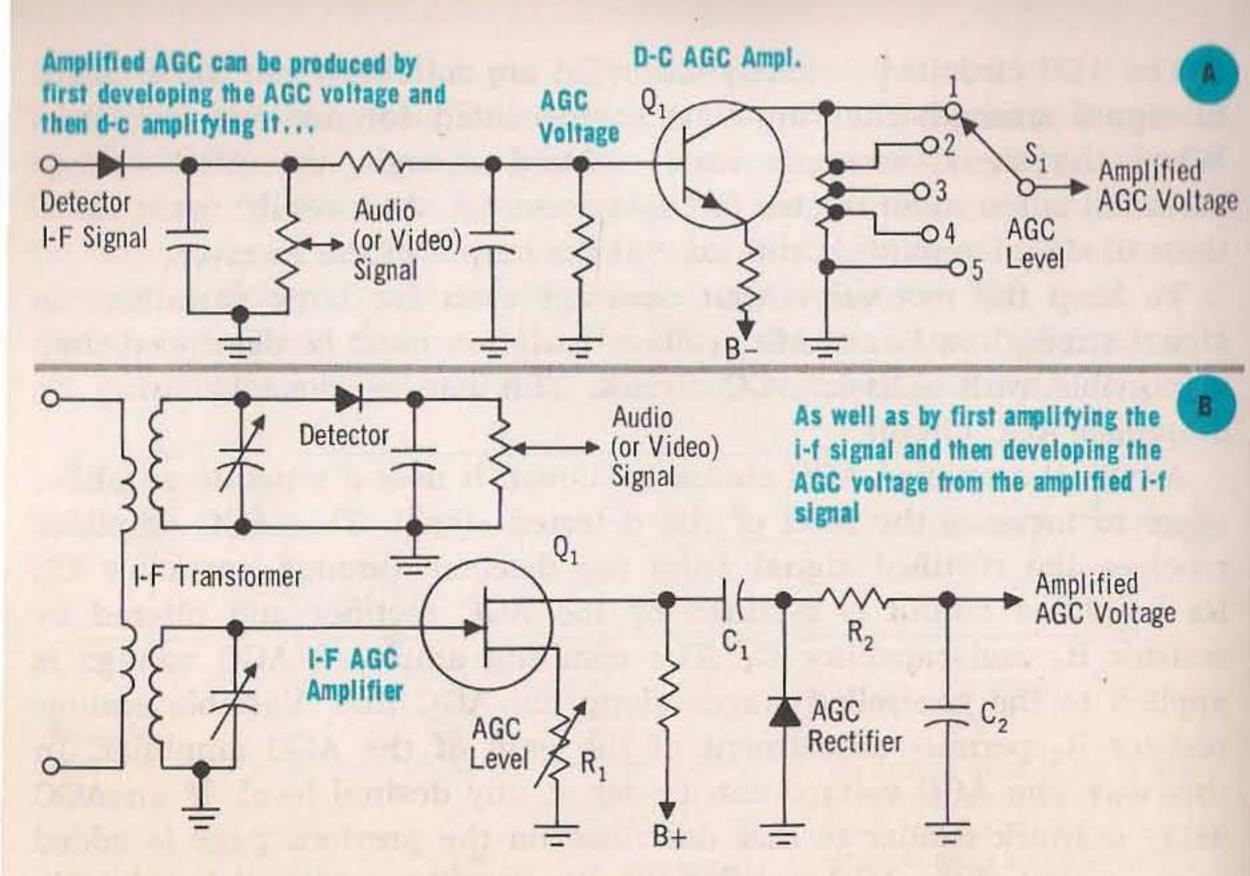
You have seen on the previous page how amplified AGC can be produced by amplifying a portion of the detector output and then rectifying and filtering the resulting amplified voltage. Other methods can also be used to produce the same type of amplified AGC voltage.
