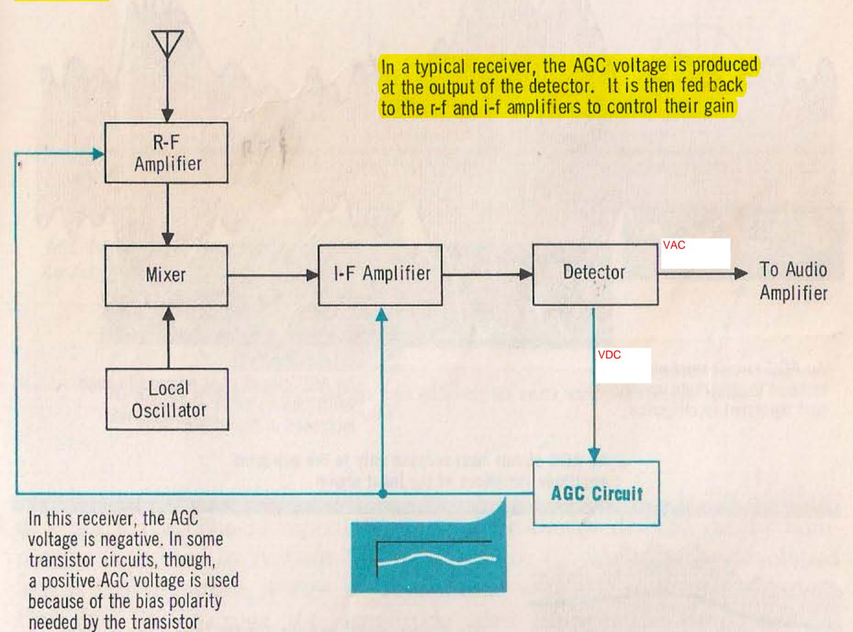
When the signal level at the receiver input increases, the AGC voltage increases a proportionate amount. Consequently, a larger bias is applied to the r-f and i-f stages, and their gain is reduced. The receiver output thus remains relatively constant, instead of increasing in accordance with the input signal strength.
