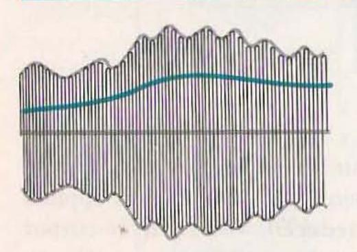
This diagram shows how the average level of the positive alternations varies with signal strength. This is the variation that produces the AGC voltage
