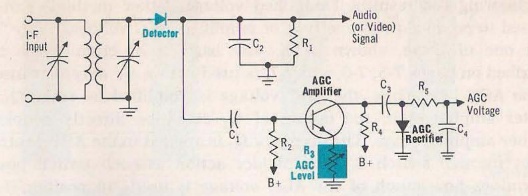
Essentially, an amplified AGC circuit contains an amplifier stage between the signal detector and the AGC rectifier and filter. An AGC level control sets the AGC action
