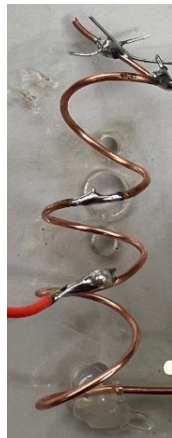
Auto-transformer from Lab 1B:
